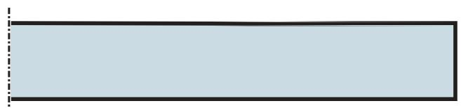
Tolerance in size according to EN 520: Width +0/-4mm, Length +0/-5mm, Thickness +0,5/-0,5mm.
